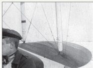
An early form of strut identification mark [86] & [87] can be seen in this close up of Rumpler C.IV 1421/17.
