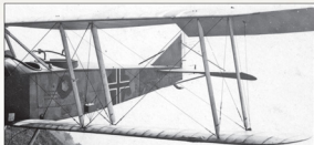
Strut and rigging detail from Lt'n Duphorn's crashed Rumpler C.IV 7620/17 (possibly from FA A 283 at Omencourt France). Note the wing attachment instructions [58] doped to the side of the fuselage, late style wing strut identification marks [90], [91], [92] & [93] and barograph [G54] + [G14] suspended between the struts. Note that rigging turnbuckles are only present where they attach to the bottom wing.
