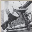
Alternative Parabellum mount and magazine fixed to an LVG style gun ring.
