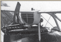
Windhoff radiator (B7 + B8) detail with shutter (A1). Note the exhaust support bracket (A50).
