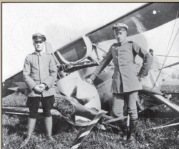
Another view of Rumpler C.IV 1449/17 B showing radiator detail, propeller laminations and 6 pointed star on nose behind propeller.
