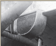
Windhoff radiator (B11 + B12) detail without any shutters. Radiators appear to have been painted the same light blue colour as the struts, although the top surface was often camouflaged.
